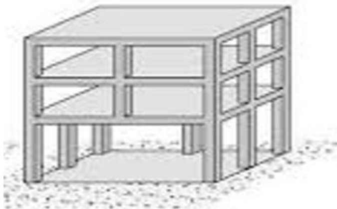
Fig. 4 stilt/Floating columns above floors
