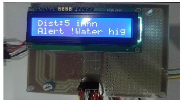
Figure 4: LCD display displaying the water level rising.
