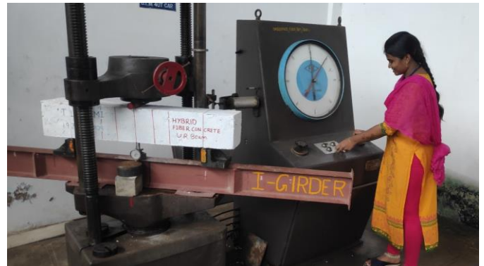
Figure 4: Testing of beam in UTM
