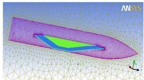
Fig 7: Meshed model of Double delta wing body without domain
