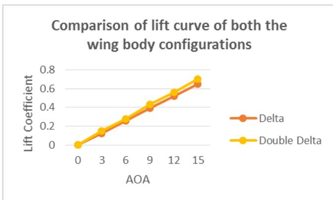
Fig 14: Lift Curve for both Delta Wing Bodies
