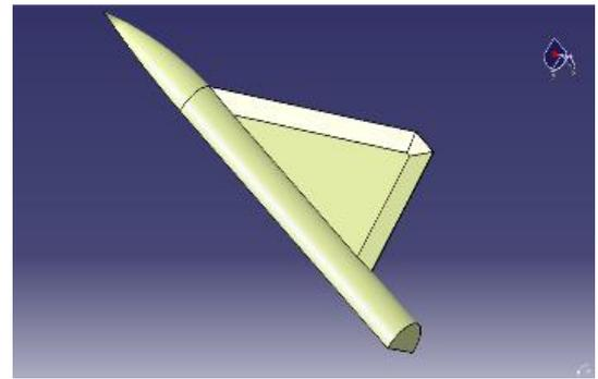
Fig 2: Cropped delta wing body (lower surface)
