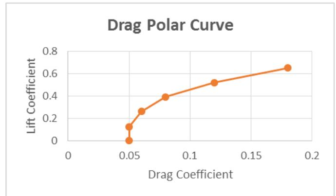
Fig 10: Drag polar Curve for Cropped Delta Wing
