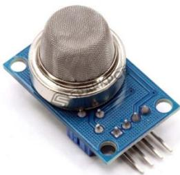
Fig.3. MQ 135/ Air quality sensor
