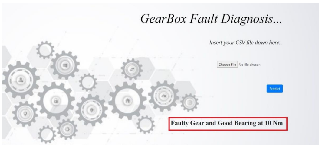
Fig 16 Predicted result for vibration data at 10 Nm condition
