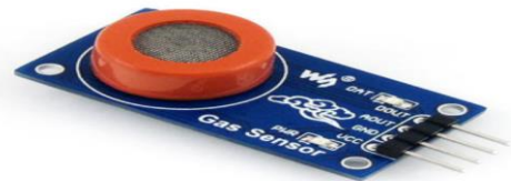
Fig 2.1.3 MQ3 alcohol sensor
