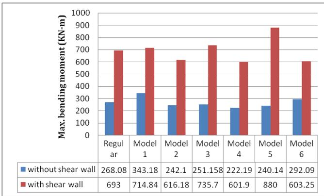
**Graph-4:** Comparative graph on maximum bending moment between different models with and without shear wall
