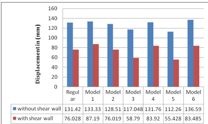
**Graph-5:** Comparative graph on displacement between different models with and without shear wall
