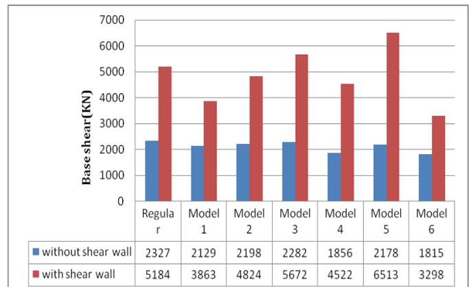
**Graph-3:** Comparative graph on base shear between different models with and without shear wall
