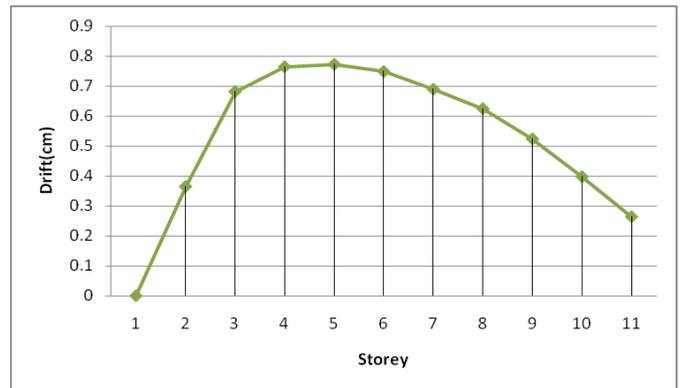
**Graph-1:** Graph between storey and storey drift of regular structure
