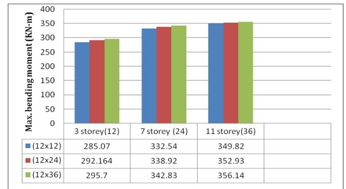
**Graph-8:** Comparative graph on maximum bending moment of vertically irregular building (stiffness irregularity) in different horizontal and vertical aspect ratio
