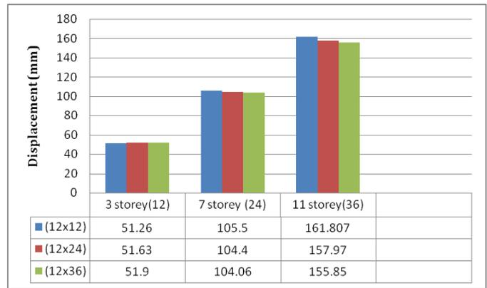
**Graph-7:** Comparative graph on displacement of vertically irregular building (stiffness irregularity) in different horizontal and vertical aspect ratio
