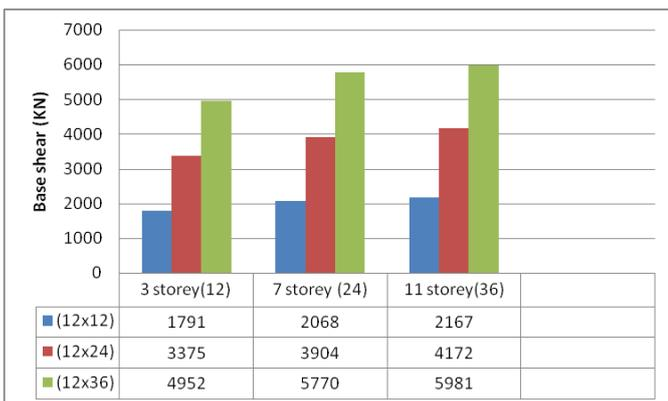
**Graph-6:** Comparative graph on base shear of vertically irregular building (stiffness irregularity) in different horizontal and vertical aspect ratio
