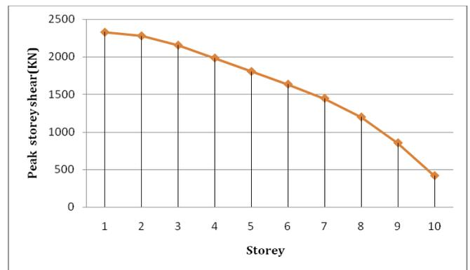
**Graph-2:** Graph between storey and peak storey shear of regular structure
