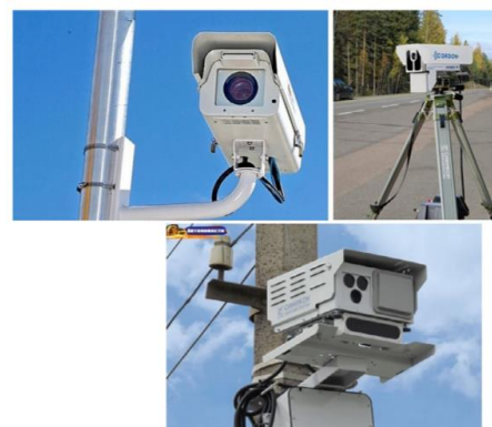
Fig 2.2.1 CCTV cameras and photoradar vehicle detectors.
