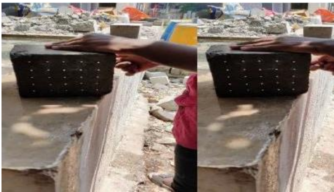
Fig -3: Transparent concrete under natural light
