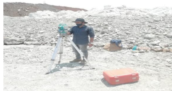
Fig.2.1 Survey data collection using Sokkia (530R/330R) Total Station
