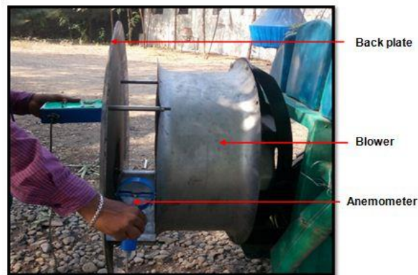
Plate 4: Measurement of blower Air Velocity
