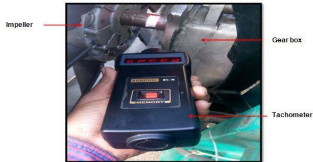
Plate 3: Measurement of blower RPM
