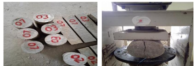
Fig 2.Split Tensile Strength Testing
