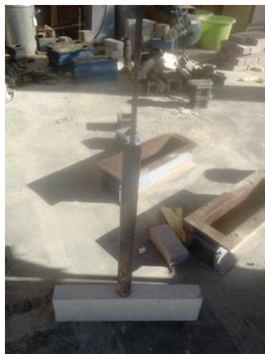
Fig. 6: Impact strength test set up for beam specimens
