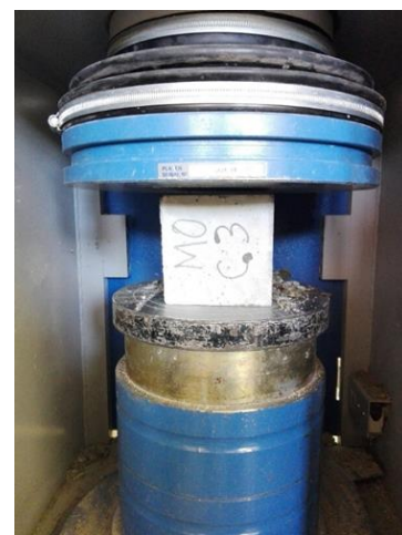
Fig. 4: Compression test for concrete cube specimens
