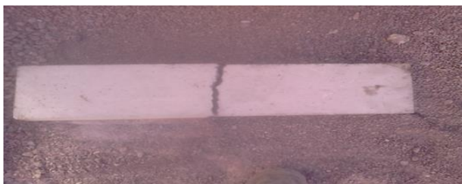
Fig. 11: Ultimate failure of unreinforced beam
