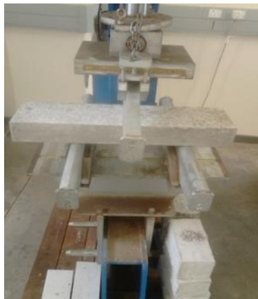
Fig. 5: Flexural strength test for beam specimens
