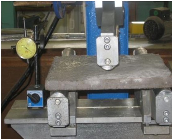
Fig. 4: Flexural strength test set-up.
