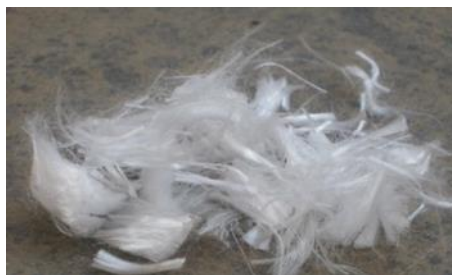
Fig. 2: Sample of polypropylene fibres
