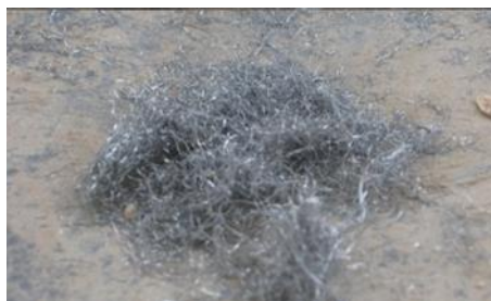
Fig. 1: Sample of steel wool fibres
