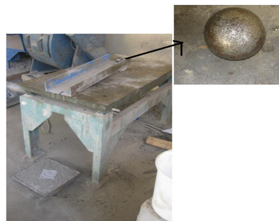
Fig. 3: Impact strength test set-up
