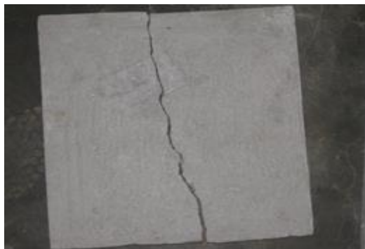
Fig. 7: Failure pattern for unreinforced slab
