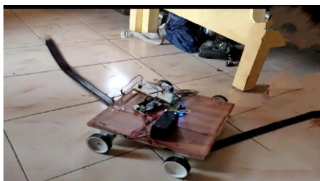
Fig -2: Robotic base programmed with Line Follower
