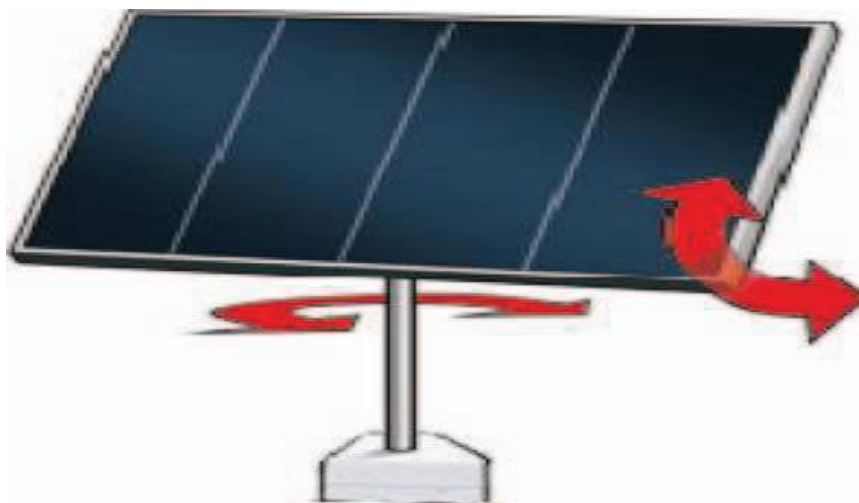
Fig. 2. Dual axis tracker
