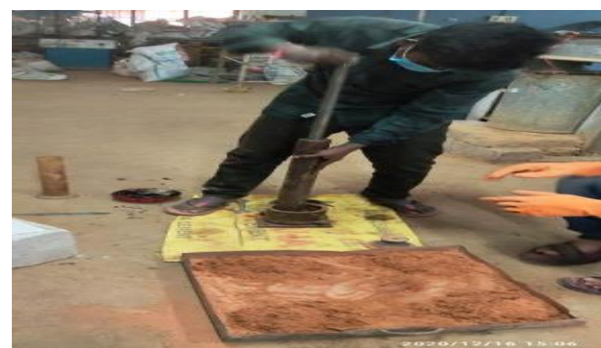
Figure-2: Modified Proctor compaction test
