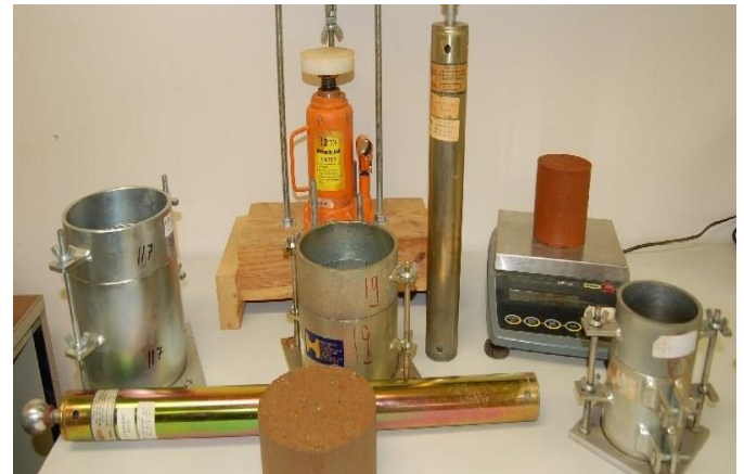
Fig-2: Compaction Test
