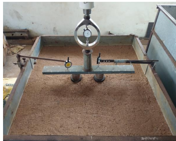
Fig. 1 Experimental set up and loading arrangement
