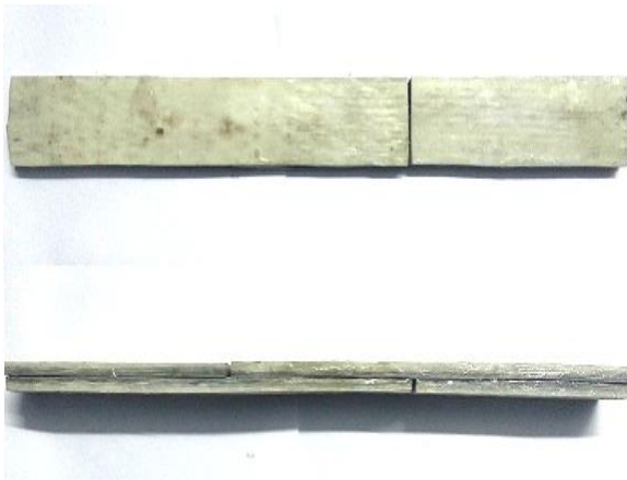
Fig. 4 Single lap GFRP joint test specimen
