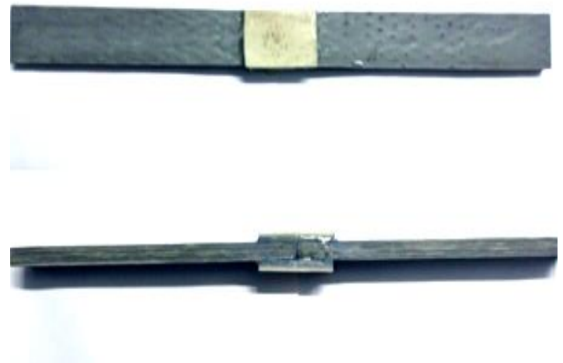
Fig. 3 Double strap GFRP joint test specimen
