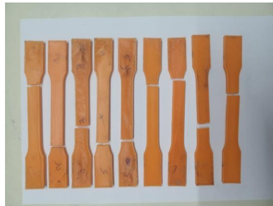
Fig 4: 3D printed specimen tensile tested in UTM
