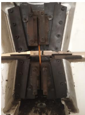
Fig 3: Mounting of specimen for tensile testing in UTM
