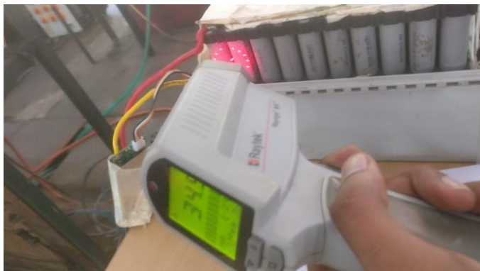
Fig -2: Measuring battery temperature using IRT
