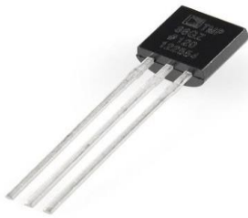
Fig -5: Temperature Sensor
