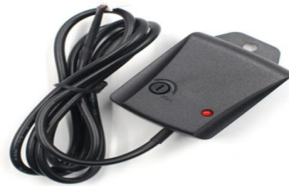
Fig -3: Vibration Sensor
