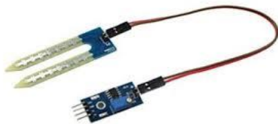
Fig -6: Oil Wetness Sensor
