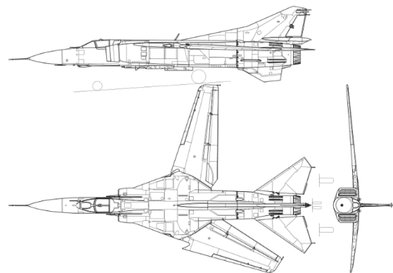
Fig. 9 Variable Geometry Wing, MiG-23
