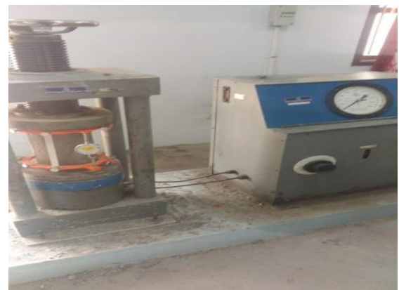
Fig.9 Testing of cylinder specimens using compression meter.
