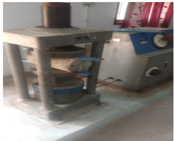
Fig.8 Testing of cylinder specimen using split tensile in compression.
