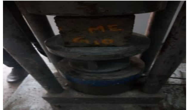
Fig 5. Testing of cube specimens in compression
