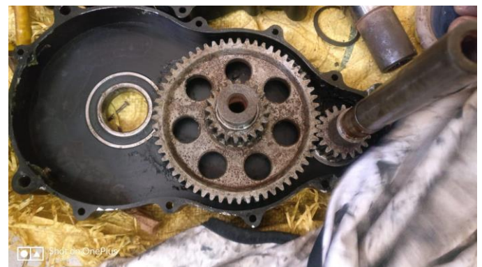
Fig. 4 2 stage reduction gearbox (11:1)
