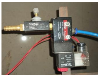
Fig -3: Solenoid Valve in prototype with Flow control valve
