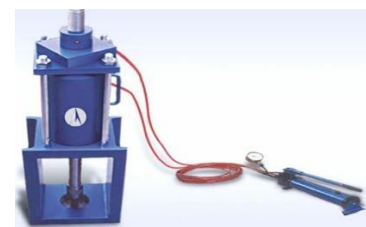
Pull Out test
