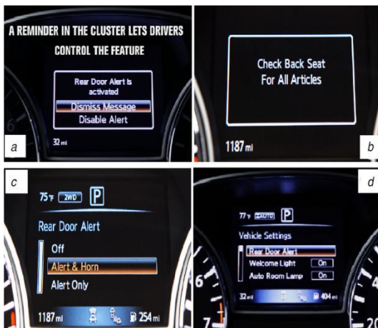
Fig. 2 Rear Door Alert system interface [2]
