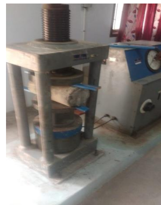
Fig: Split Tensile Strength Test of Specimen
