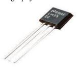
No external calibration or trimming is required for the LM35 system to deliver typical precisions of  $\pm 1/4$  °C at ambient temperature and of  $\pm 2/4$  °C over the full range of -55°C to 150°C. Low-performance impedance, linear output and accurate inherent calibration make it particularly easy to interface with or control the circuitry. The standard body temperature is between 97.5 and 99.7 degrees Celsius. If the temperature ranges from 100 to 103 degrees FF, this shows viral fever.
