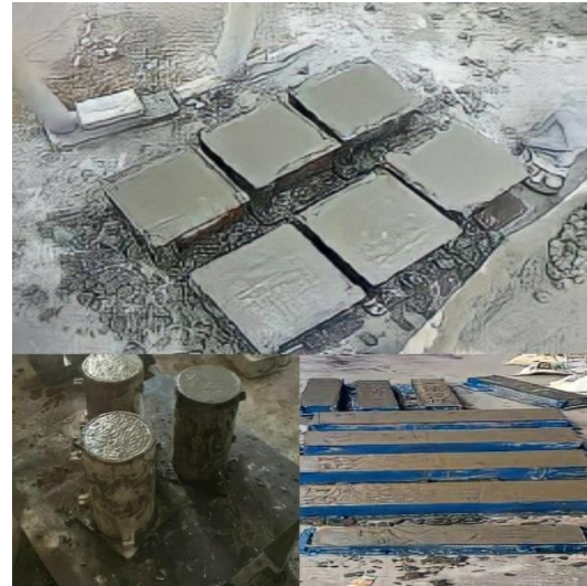
Fig 2: Casting of specimens
