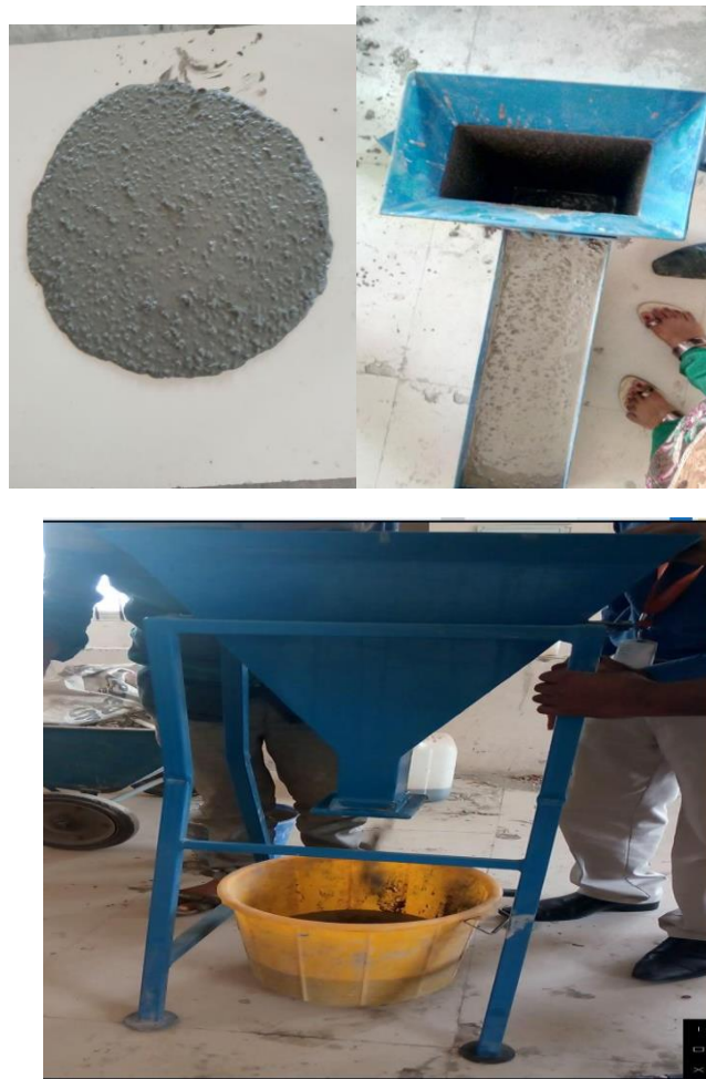
Fig 3.2 Slump flow test L-box test, V-funnel test
