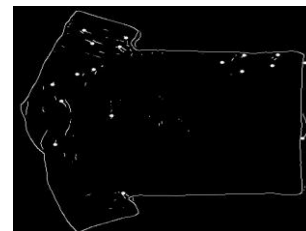
Figure 13: Incorrect corner identification due to lot of wrinkles
