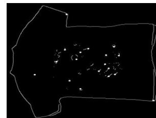
Figure 12: Incorrect corner identification due to design
