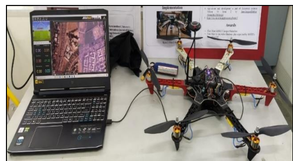
Fig -2: The proposed system (Hex copter with computer interface)
