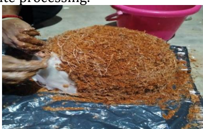
Fig -2.6: Sample preparation by wet hand lay-up process
