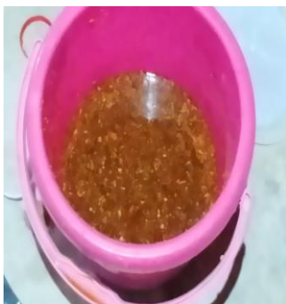
Fig -2.5: Surface Treatment with NaOH
