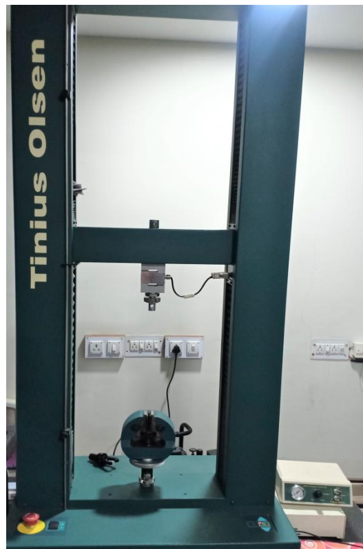
Fig -7: Universal Testing Machine set up
