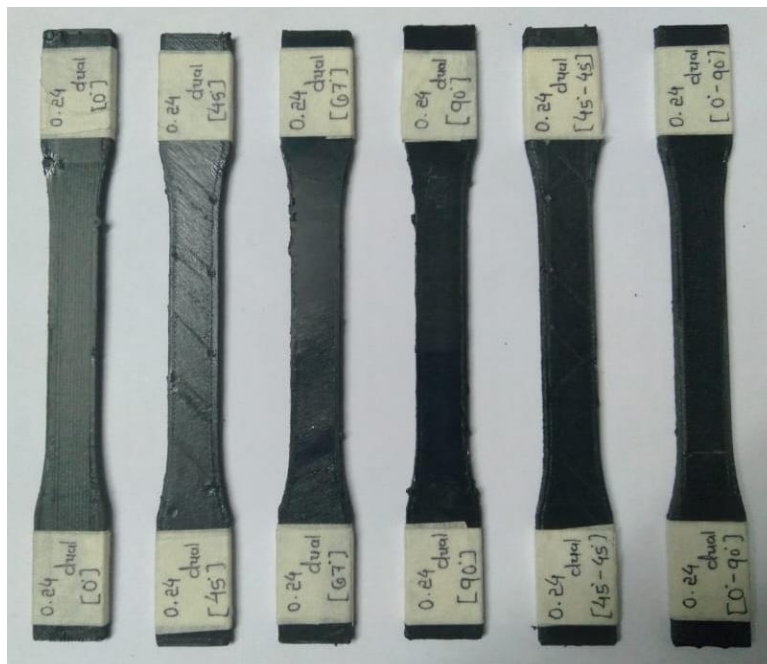
Fig -8: One set of dual FDM printed specimens at 0.24mm layer thickness at variable raster angle
