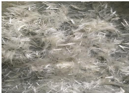
Fig -2.1: Anti-crack high dispersion glass fibers
