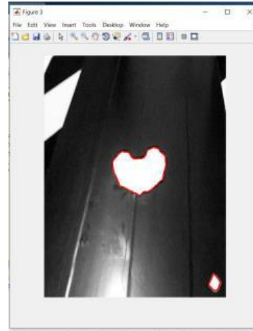
Fig -7: Pothole Boundary Identification
