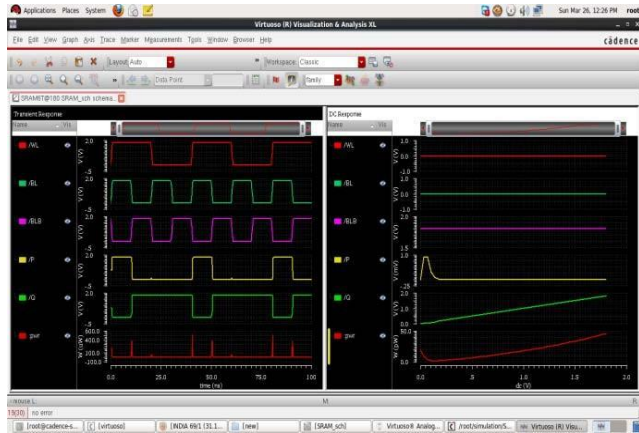
Fig.2 Transient and DC response of 6T SRAM
