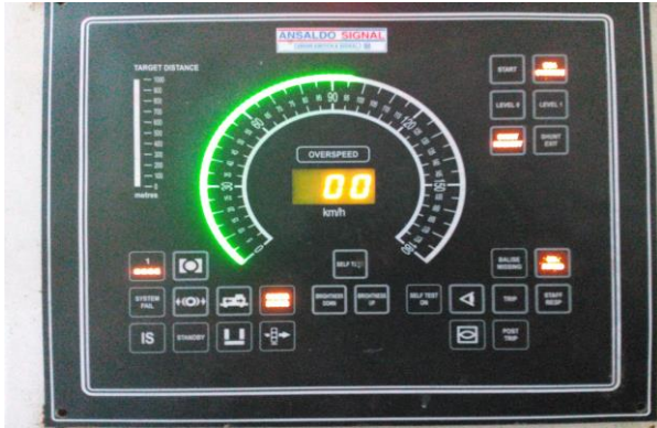
Fig-4: DMI Displaying the alerting message.
