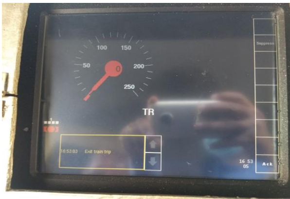
Fig-5: After applying brake the DMI Displaying to EXIT the Train trip.
