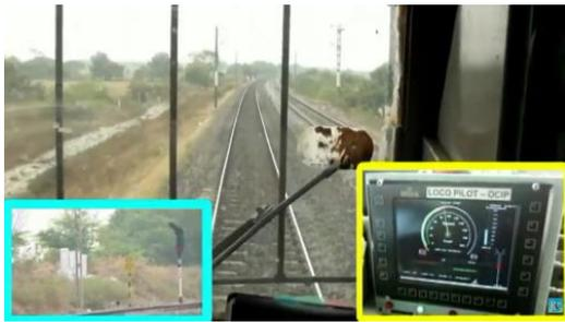
**FIG -3:** The System Indicates that there is Red Signal on the Track
