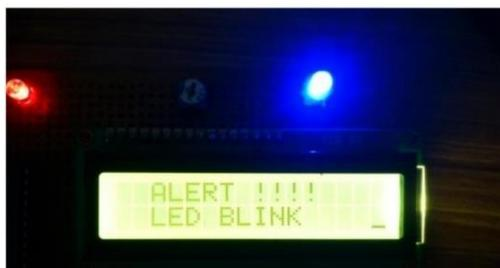
**FIG -6:** Alert Message in the LCD Display with Flash Light and Alarm
