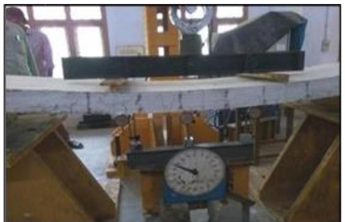
Fig. 4: Test set up for Static loading under loading condition
