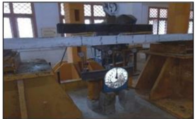
Fig. 3: Test set up for Static loading
