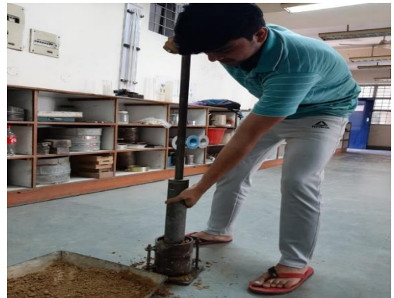
Fig.6 Modified Proctor compaction test
