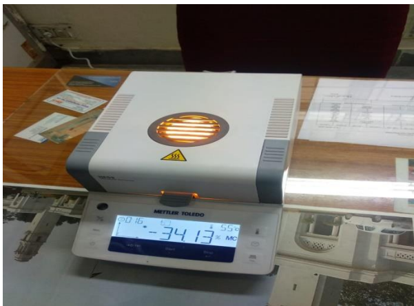
Fig.11 Determination of moisture content
