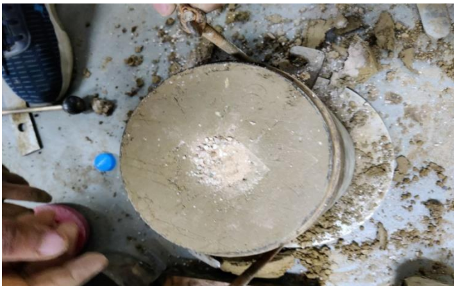
Fig. 14 CBR mould prepared with granular pile
