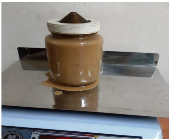
Fig.5 Test for Specific gravity of clay.
