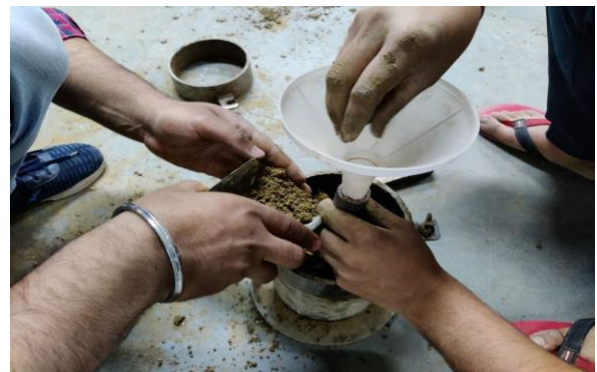
Fig. 16 CBR mould prepared with granular pile encased with non-woven geotextile
