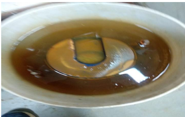
Fig. 15 CBR mould in soaked condition
