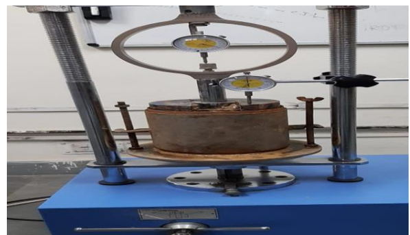
Fig. 17 Testing of sample with granular pile encased with non-woven textile
