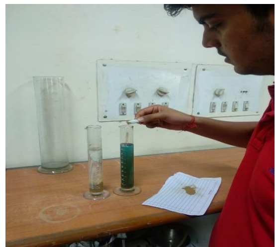
Fig.7 Free swell index test for clay
