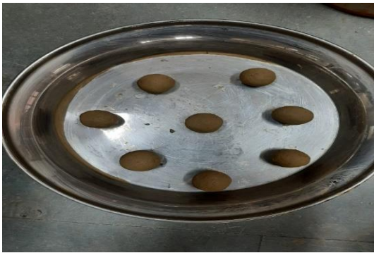
Fig.3,4 Determination of liquid limit and plastic limit
