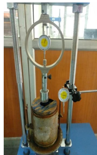
Fig. 12, 13 CBR test for pure clay soil
