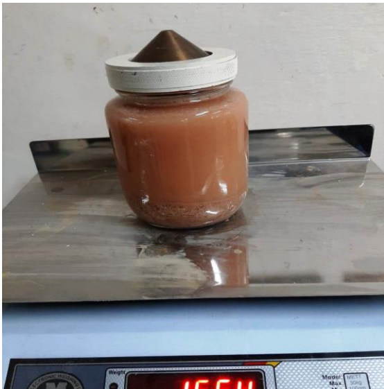
Fig.9 Specific gravity for granular material
