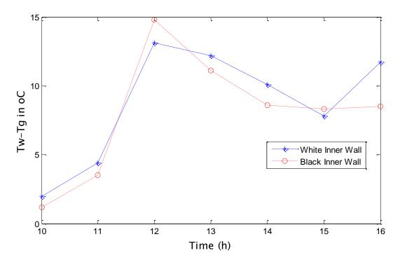
Fig 3 Difference between Water Temperature and Glass Temperature (T<sub>w</sub>-T<sub>g</sub>) with respect to time for Black Inner Wall and White inner wall solar still for a typical day of month May-June 2014
