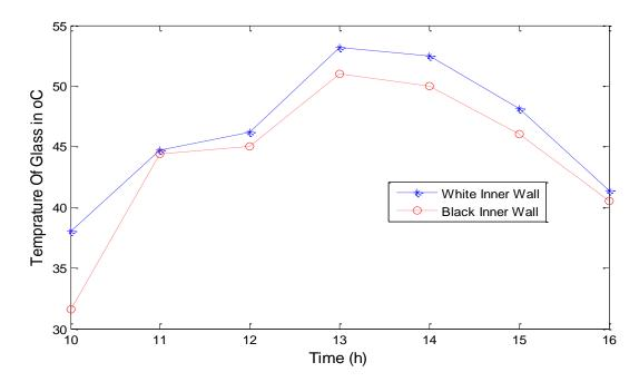
Fig 2 Hourly Variation of Temperature of Glass for Black Inner Wall and White inner wall solar still for a typical day of month May-June 2014
