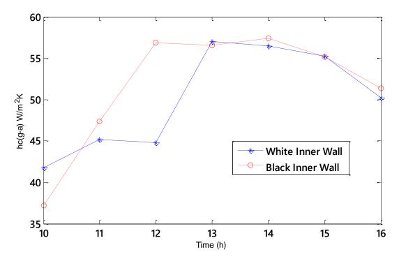
Fig 7 variation of convective heat transfer coefficient between water and air with respect to time for white and black inner wall
