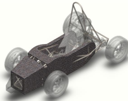
Fig-2: Installed monocoque with assembly
