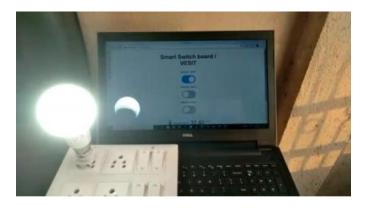
We have made a website to control the switches and display temperature of the room. Three appliances can be connected to this switchboard and a temperature sensor is also connected. At present we can operate the switchboard using this website from anywhere within the WIFI range but we can also use cloud services to operate it from anywhere in the world by a monthly subscription to their services.
