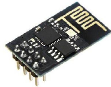
Figure 3: ESP-01S that contains TCP/IP socket
