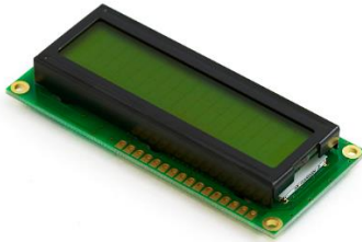
Figure 6: LCD Display that shows the locker open/close status.
