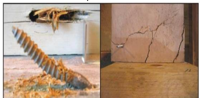
Fig. 9: Failure of push-out specimens
